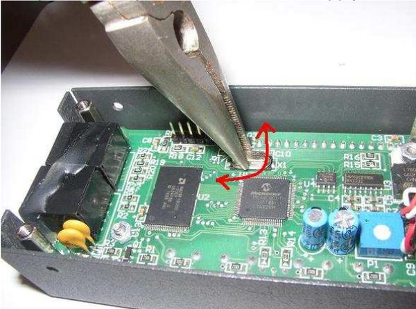
17- Once the quartz is removed, clean up the pads with the welder and add a little amount of soldering.
