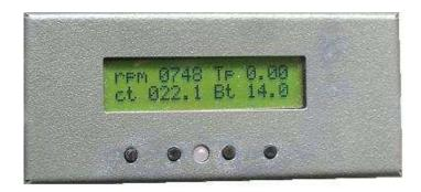
In this working mode the NANOCOM starts automatically to read and shows the four main fuelling parameters with the frequency of four times per second as a board's instrument. The Nancom turns itself to standby a few seconds after you turn off the ignition.
